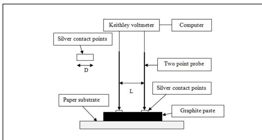
Fig. 1: Computerized two point probe diagram to characterize I-V curve of graphite paste electrodes with silver conductive paint.
