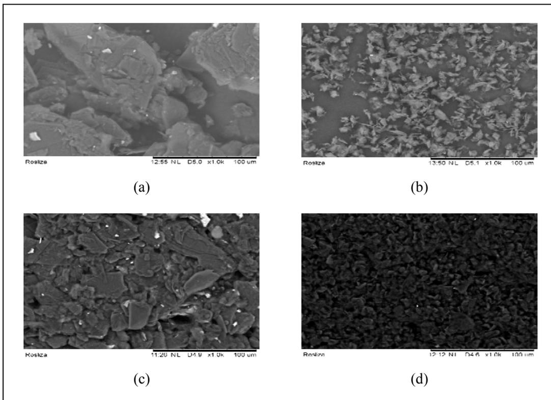
Fig. 2: FE-SEM micrographs of (a) natural graphite powder, (b) micronized graphite powder, (c) natural graphite paste electrode, and (d) micronized graphite paste electrode.
